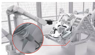
Door welding inspection
